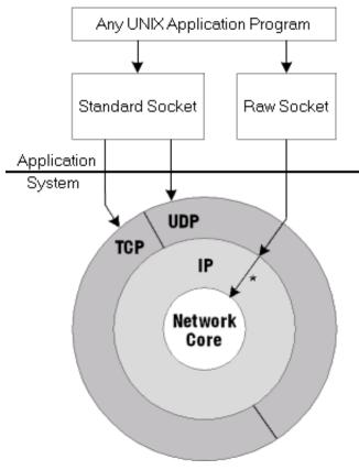
Circa 1981 — The Computer Systems Research Group (CSRG), at the University of California at Berkeley, first mated the Unix operating system to the Internet. This was done by implementing the Internet protocols and creating a so-called "TCP/IP Stack" for Unix. This is shown as concentric regions in the diagram to the Jeft.
